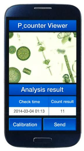
Ballast water Performance Standard (D-2) in the Ballast Water Management(BWM) Convention indicates that less than 10 viable organisms with less than  $50\mu m$  and greater or equal to 10 µm should be found in 1 milliliter of ballast water. Reinforcing the regulation requires a precise monitoring tool for minimal impact in oceans.
