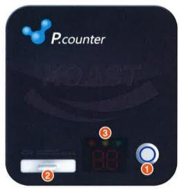
Simply 1 turn it on, 2 put the filter in and (3) read the result.
