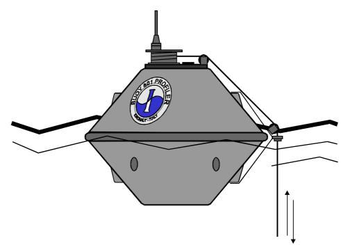
The acquired data is buffered by the Controller, awaiting the 'calls' from the Land-Based Station. Once the communication is established, the buffered data flows in CRC controlled messages from the Buoy to the Land-Based Station. Communication occurs at programmable time intervals.
